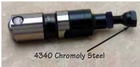
4340 CHROMOLY STEEL SCREW, WITH OIL HOLE, TO FEED TOP END.
